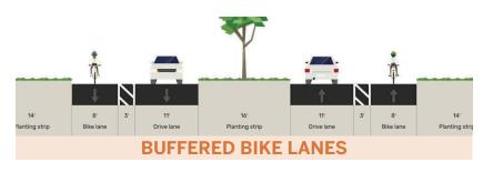
Bike facility constructed with mill and overlay
