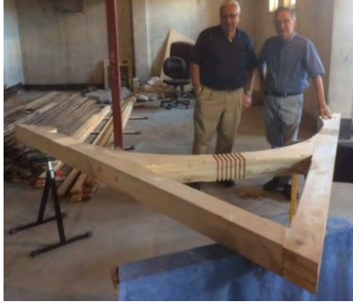
2014 Three-piece brackets crafted and assembled.
