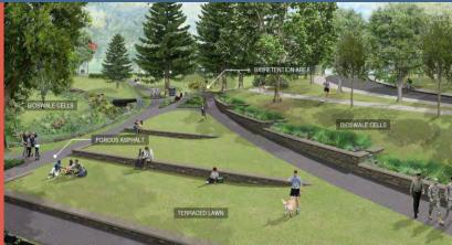
Stormwater management components are integrated with park design features
