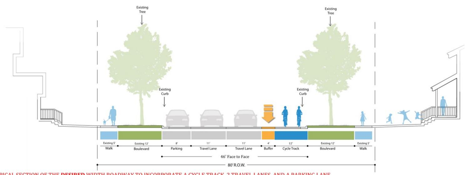
TYPICAL SECTION OF THE **DESIRED** WIDTH ROADWAY TO INCORPORATE A CYCLE TRACK, 2 TRAVEL LANES, AND A PARKING LANE
