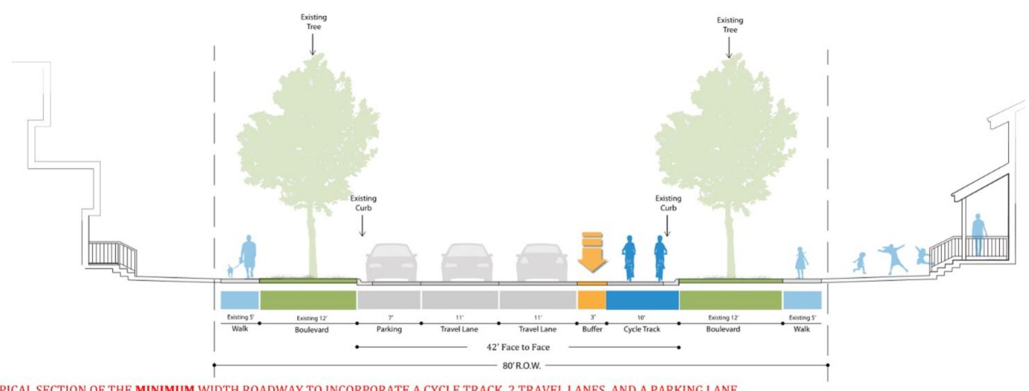
TYPICAL SECTION OF THE MINIMUM WIDTH ROADWAY TO INCORPORATE A CYCLE TRACK, 2 TRAVEL LANES, AND A PARKING LANE
