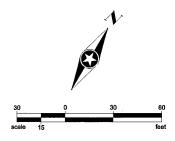
ORIENTATION OF THIS BEARING SYSTEM IS BASED ON THE RICE COUNTY COORDINATE SYSTEM (NAD 83 -1996 ADJ.) WHEREIN THE NORTHWESTERLY LINE OF LOT 1, BLOCK 1, CLINTON HEIGHTS BEARS N 45°24'22" E.
