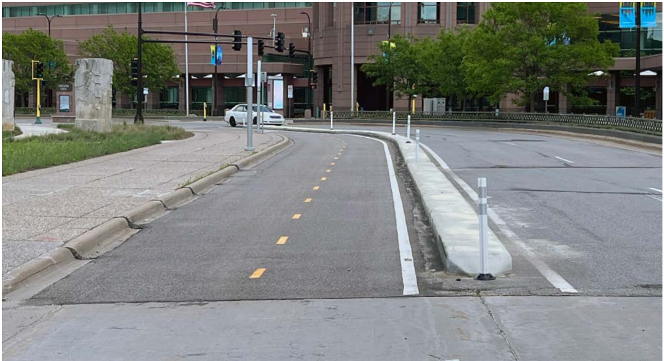
Two way separated bikeway example with concrete bike buffer in Minneapolis
