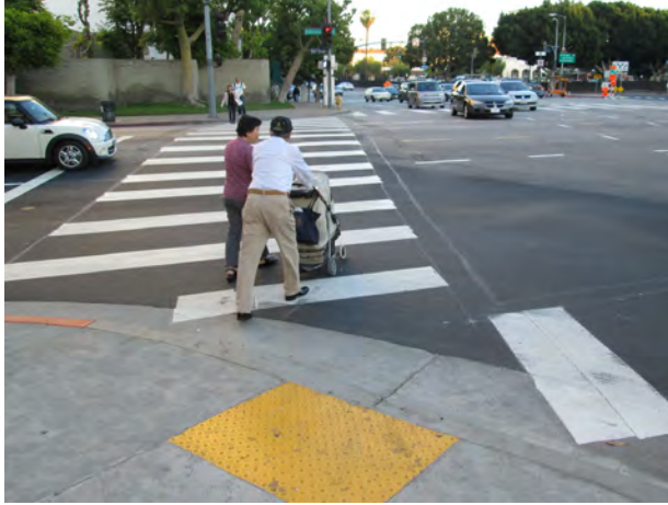
Not recommended: Diagonal curb ramp configuration.
