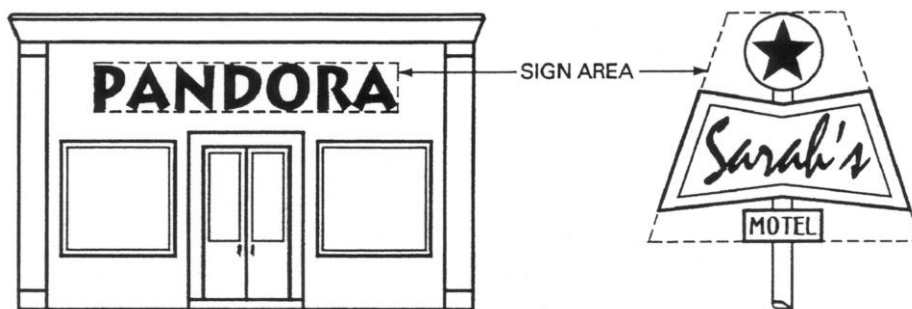
Figure 6-1: Illustration of how sign area is calculated.
