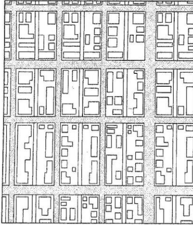
Figure 9-2: Illustration of Grid Street Pattern.
