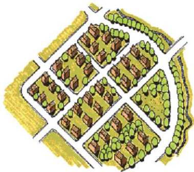
Figure 9-3: Illustration of a Modified Grid Street Pattern.
