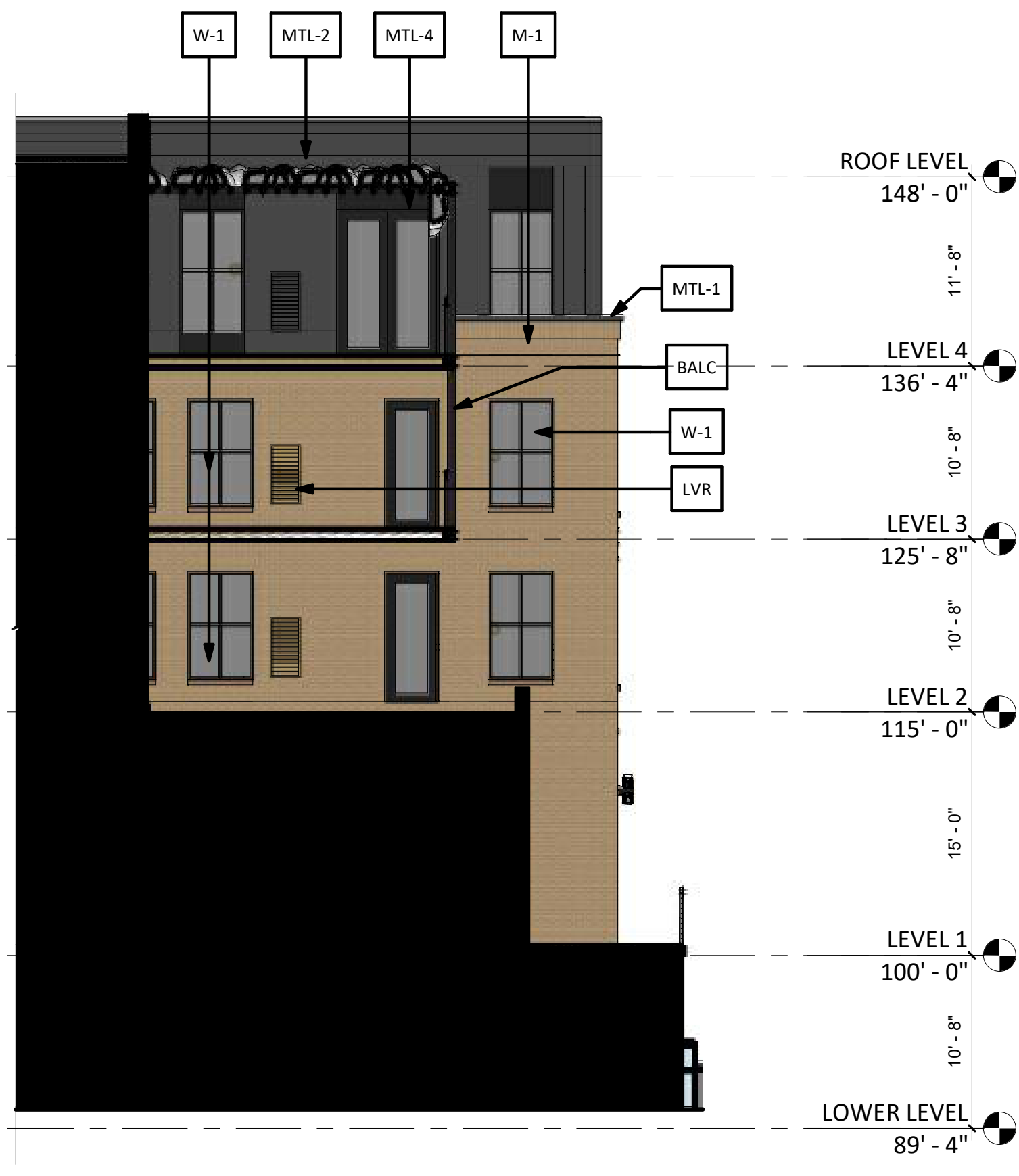
4 NORTH ELEVATION - SOUTH TERRACE MP3.1 1/8" = 1'-0"
