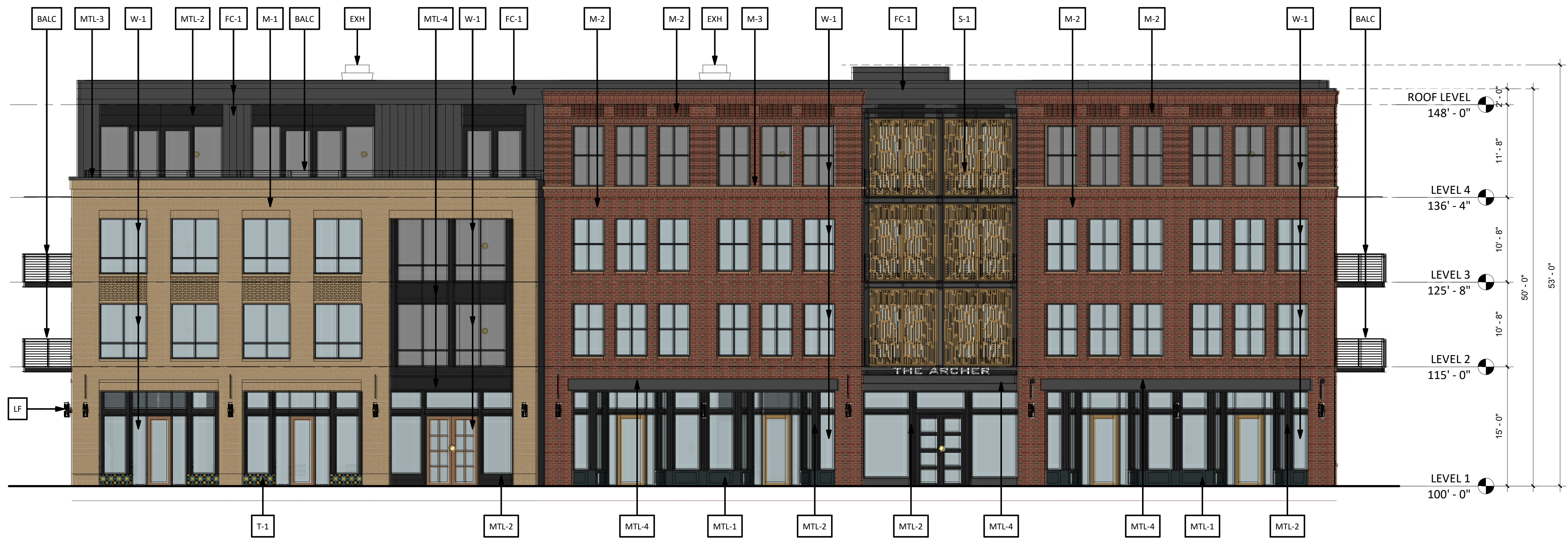
1 EAST ELEVATION MP3.1 1/8" = 1'-0"
