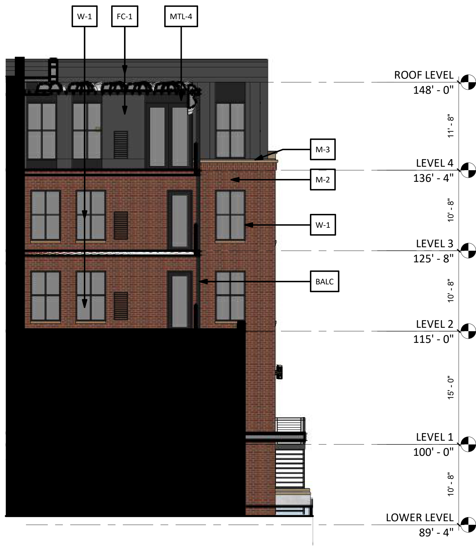
3 NORTH ELEVATION - NORTH TERRACE MP3.1 1/8" = 1'-0"
