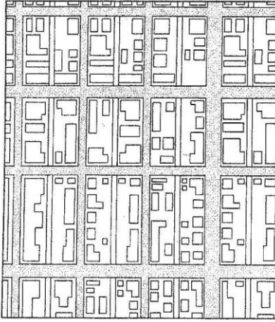
Figure 9-2: Illustration of Grid Street Pattern.
