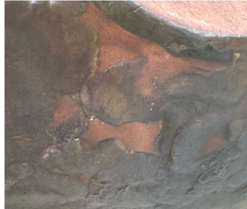
Figure 1. Red areas are copper under the phos-copper
