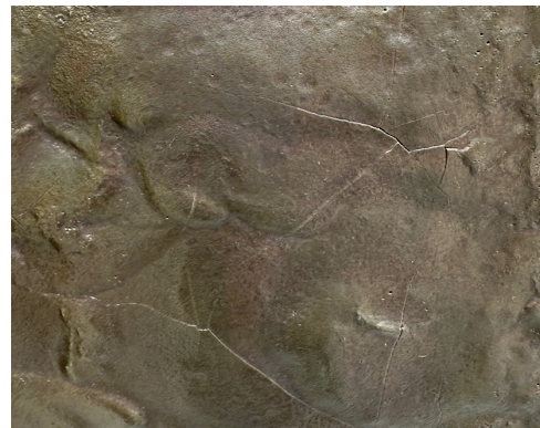
Figure 2. Original cracks from fabrication
