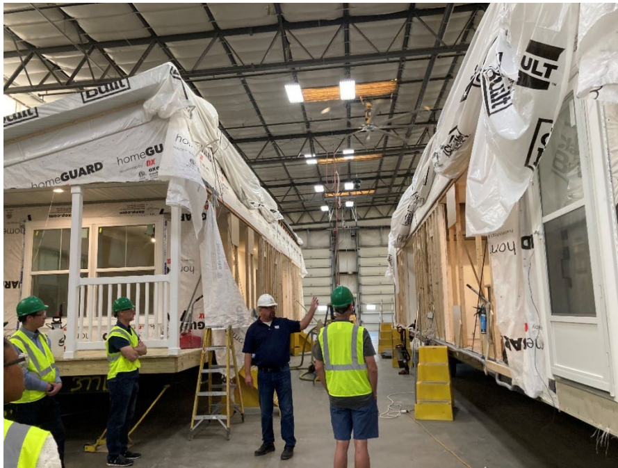
Two sections of the same Schult manufactured home next to each other (they will be transported separately and put together on-site)
