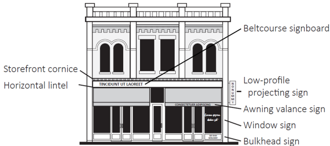
Figure 6-3: Illustration of where signs are historically attached to buildings in the downtown historic district.
