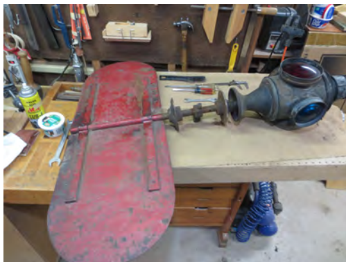
2017 Mechanism needing cleaning
