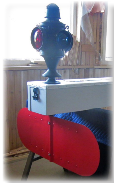
The donated order board was restored. A 1896 photo shows an order board mounted on the exterior of the station master bay. It was used by the station master to communicate with an engineer of an approaching train.
