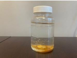
Pictures above are from fire hydrants when they were in operation. Shows the iron in the system.
