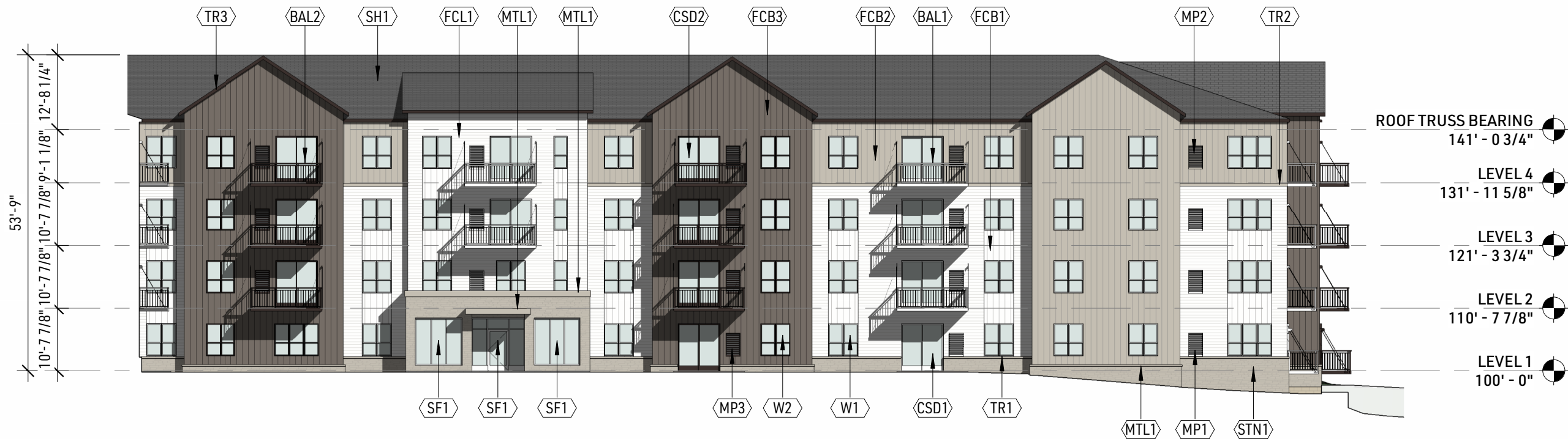
1 ELEVATION - NORTH - MAIN ENTRY 1" = 20'-0"
