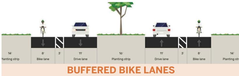
Bike facility constructed with mill and overlay
