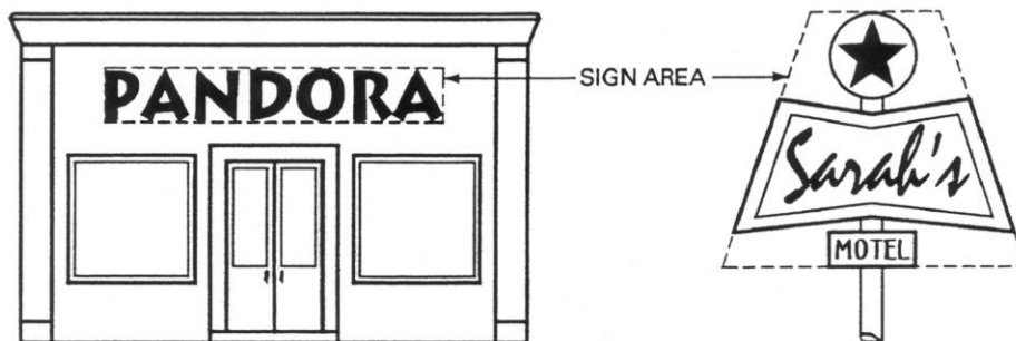
Figure 6-1: Illustration of how sign area is calculated.
