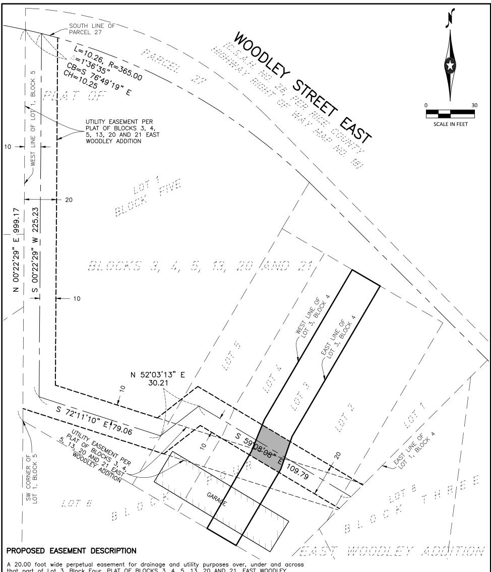
A 20.00 foot wide perpetual easement for drainage and utility purposes over, under and across that part of Lot 3, Block Four, PLAT OF BLOCKS 3, 4, 5, 13, 20 AND 21, EAST WOODLEY ADDITION, according to the recorded plat thereof, Rice County, Minnesota, the centerline is described as follows:
